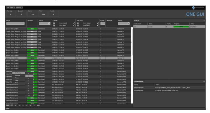
Furthermore ONE GUI allows connecting to various processing farms at the same point in time. For instance it can be used as central monitoring and operating interface to transcoding farms from different vendors.
